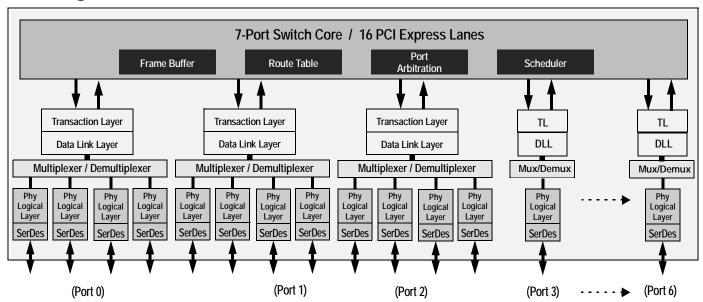
Figure 1 Internal Block Diagram
